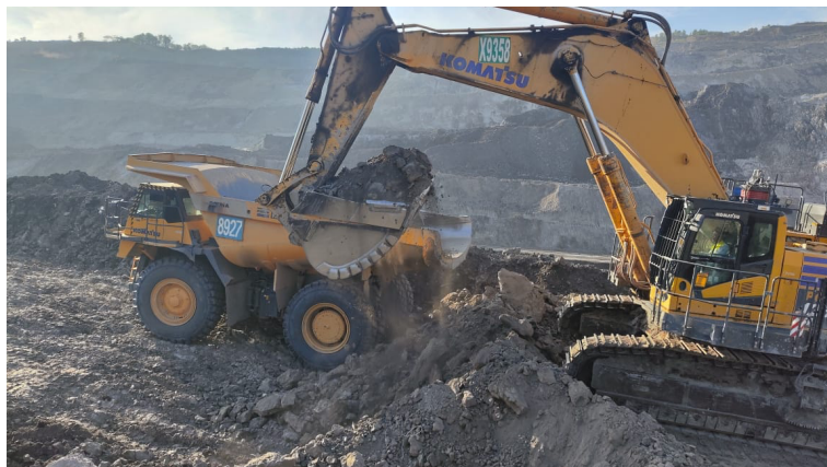
Gambar 5. Tinggi jenjang excavator loading material ripping
