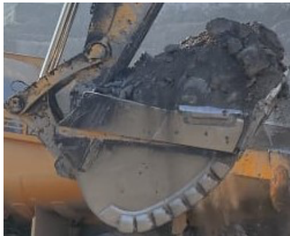
Gambar 3. Aktual isian bucket excavator
