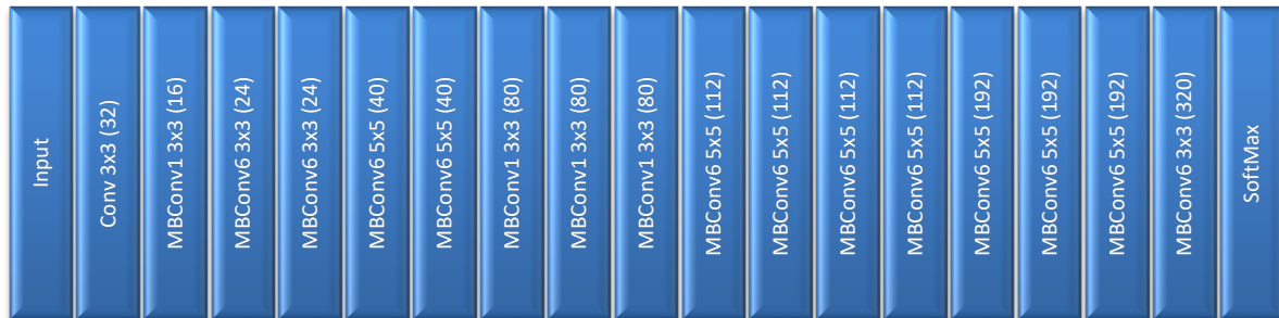
Figure 4. The architecture of Efficient-Net
