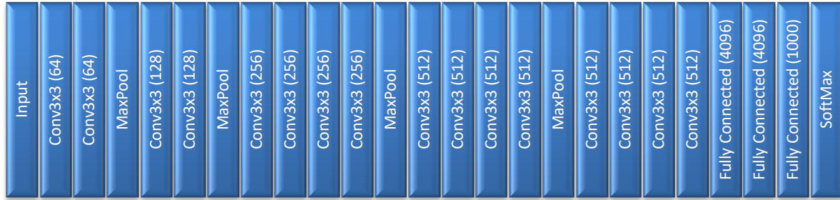
Figure 3. The architecture of VGGNet-19
