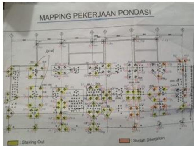
Gambar 12. MappingPengecoran Bore Pile
